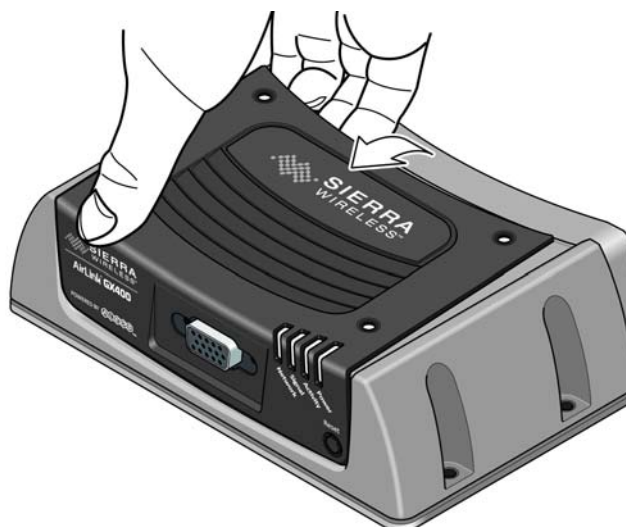
Figure 2-8: Tilting the cover (I/O X-Card installed)
