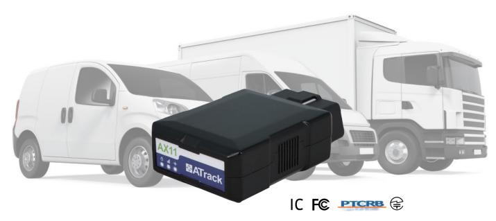
AX11 is a 4G LTE Cat.1 / Cat. M1 GPS tracking unit with OBDII interface and plug-n-play installation. Featuring OBDII, J1939 and J1708 data acquisition, optional bluetooth connectivity, driving behavior event management, and user-defined reports, AX11 is an ideal solution for usage based insurance, car rental, fleet management of both passenger vehicles and heavy-duty trucks.
