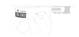
Once the device is connected and receives power, the LEDs on the front of the device start blinking then turn solid once completing the actions below.
